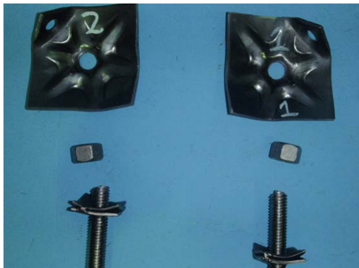
Figure 2. Y18 x 1.8 m Long Roof bolt assemblies after the test.
