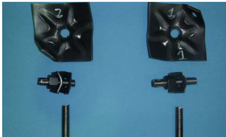
Figure 2. Y16 x 1.2 m Long Roof bolt assemblies after the test.
